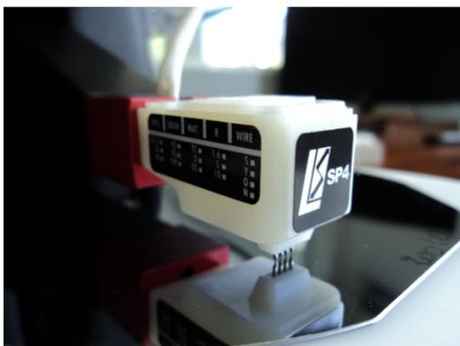
The SP4 is a low-cost disposable and inline probe made of Delrin and compatible with a majority of most applications. Several choices are available for configuration to your specific application. Three spacings are available 1, 1.27 and 1.6 mm. The three pressures available are 45, 85, and 180 grams. Tips are made of Tungsten Carbide or Osmium and a choice of 40, 125 or 254  $\mu\text{m}$  radius.
